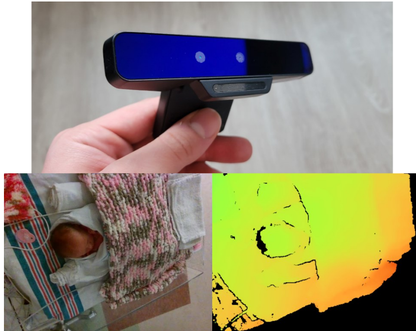
Figure 10: Intel RealSense SR300 with examples of RGB and color-mapped Depth patient data
