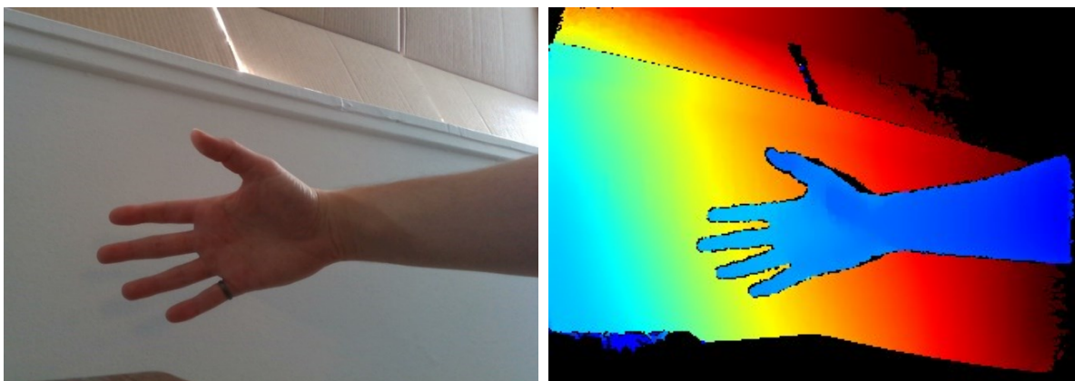
Figure 3: RGB and depth image of the same scene taken using the Intel RealSense SR300
